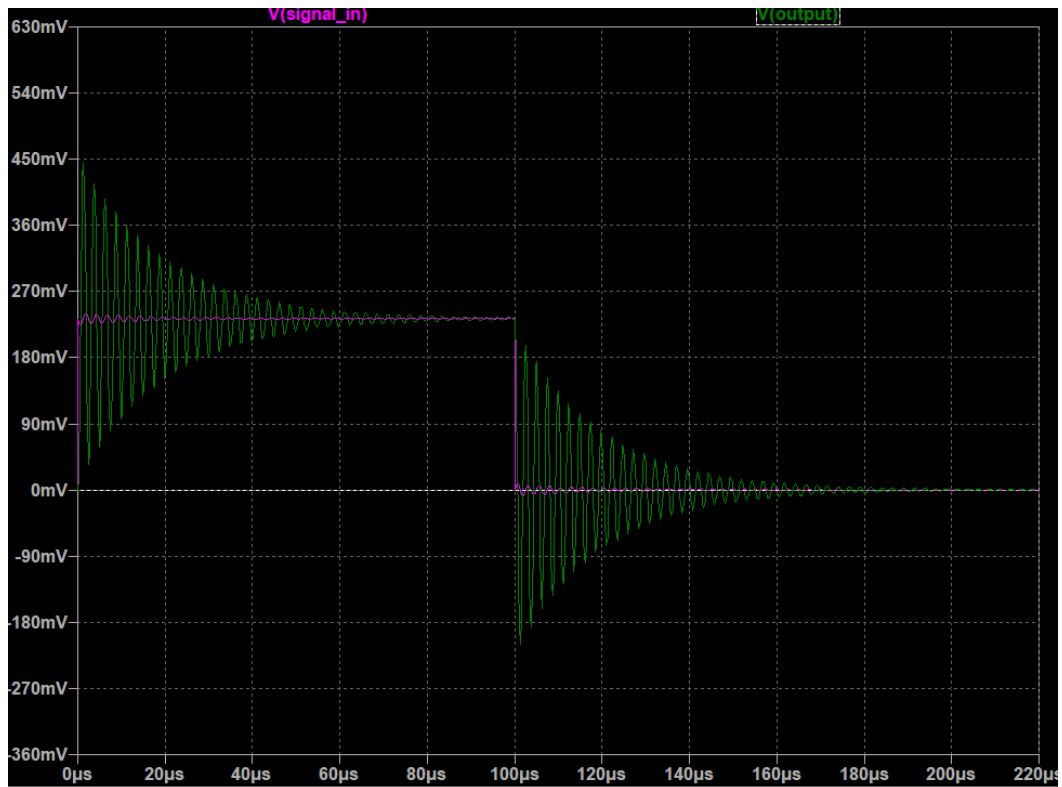
Figure.7: Step Function Response of the Capacitor, LTspice simulation
