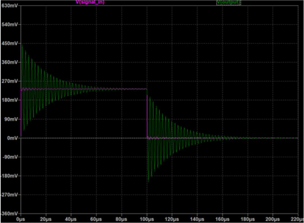
Figure.7: Square Wave Response, LTspice simulation, from Preliminary Report
