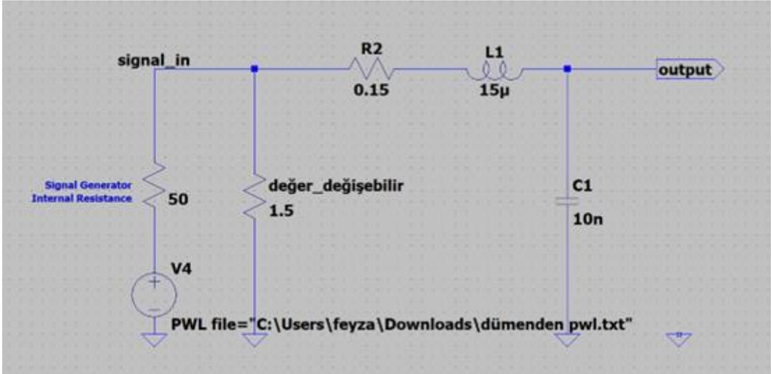
Figure.6: LTspice schematic of the circuit, from Preliminary Report
