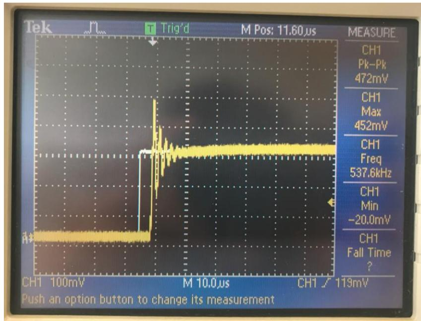
Figure.9: Square Wave Step Function Input and the Voltage of Capacitor
