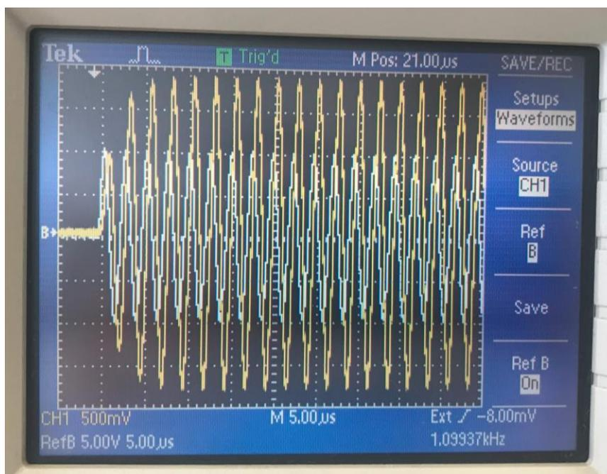
Figure.10: Sinusoidal Wave Pulse Input and the Voltage of Capacitor
