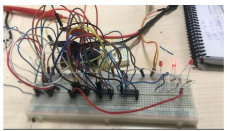
6- Finally, I added LEDs and resistors (560  $\Omega$ ) to show my circuit is working according to my truth table.
